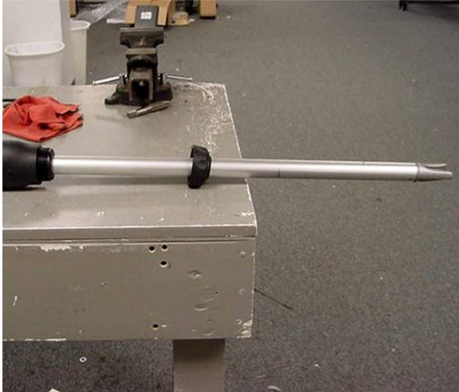
5. Use the punch and hammer to drive the spring pin into the body of the tube. The pin must be clear of the push/pull tube.
