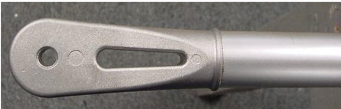
2. Center punch and drill a 1/8" or 5/32" hole (depending on the size of your spring pin) through the push/pull tube and front mount.
