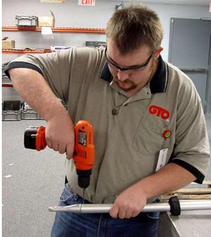
3. Insert the spring pin in this hole and tap it in until it is flush with the surface of the push/pull tube.
