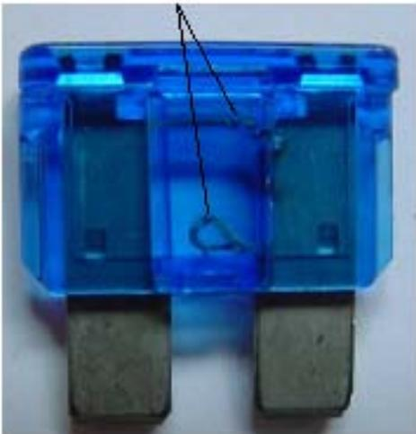
If the wire is intact, the fuse is good.
