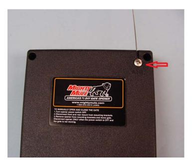
Check to make sure that the metal antenna is not broken. If broken the antenna would need to be replaced.
