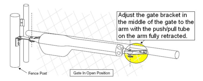
Make sure the gates are in the fully open position and the arms are fully retracted.
