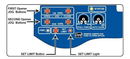
With the gates in the desired closed position PRESS and HOLD the SET LIMIT button until the alarm and set limit comes on. Then release the button.
