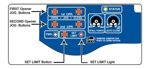
Press and HOLD the 1st Openers CLOSE button on the control board and be prepared to RELEASE the button when the gate reaches the desired close position. Use the JOG OPEN and CLOSE buttons to "fine tune" gate position if necessary
